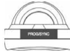
\*If your sensor is correctly aligned the RED LED on the Sensor will come on SOLID RED changing to FLASHING RED. You should see a reading on the top line of your display within 2 minutes.
